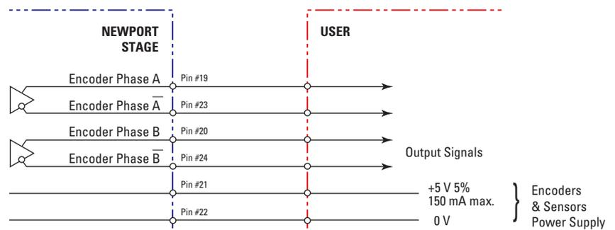
“Encoder” are “differential pair” (type RS-422) type output signals. Using these signals permits a high immunity to noise. Emission circuits generally used by Newport are 26LS31 or MC3487. Reception circuits to use are 26LS32 or MC3486.
