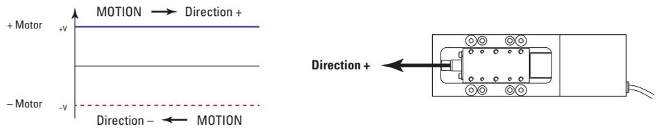
In the above drawings, + Motor signal is referred to - Motor signal.
